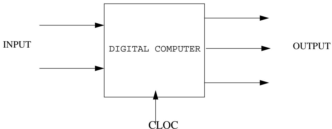
The machine changes its state at discrete “points” in time. The clock determines when state changes can happen.
